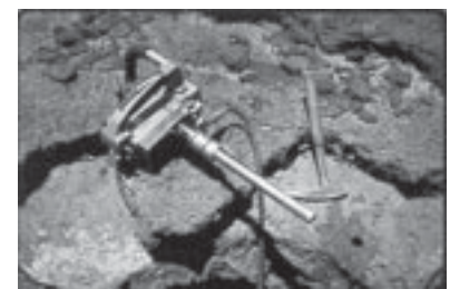
Tools of the trade: A core sample drill and rock hammer (Photo: Sharon Ringsven)
